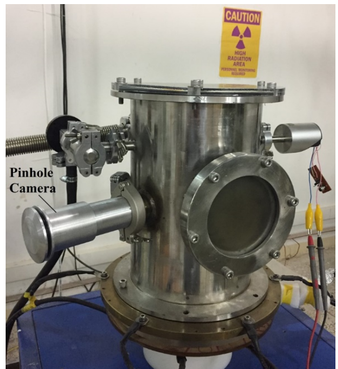
Figure 2: Plasma focus device and assembled pinhole camera which installed on the wall of the chamber.
