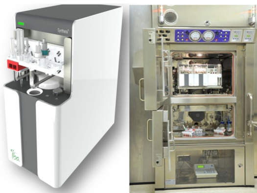
Figure 2: The synthesis module and Hot-cell for FDG.
