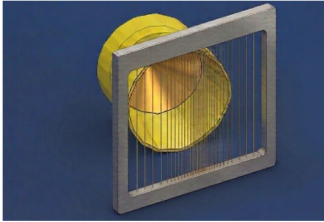
Figure 13: CAD model of the SEM grid Faraday cup diagnostic assembly used for beam profile measurements.
