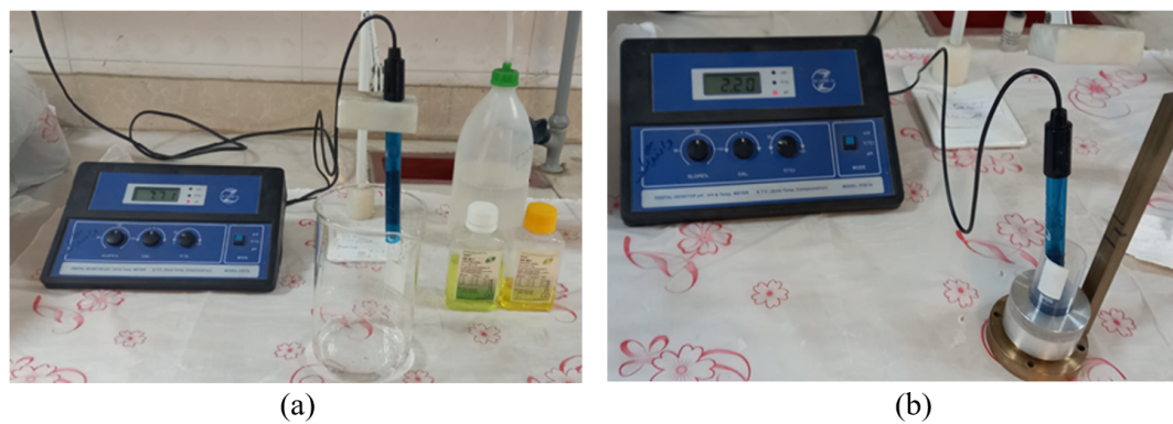
Figure 4: (a) pH meter calibration and (b) sample solution pH adjustment.
