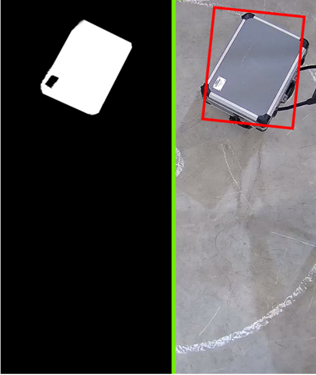
Figure 6: The color segmentation and detection of luggage were achieved using image processing techniques. The right image displays the original image with the detected object outlined in a red bounding box, while the left image demonstrates the separation of target pixels from the background.
