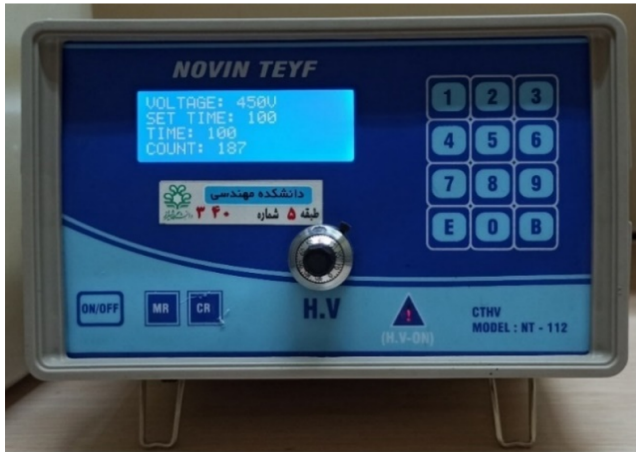
Figure 4: Setup and measured count with the Geiger-Muller detector on day 10 of the experiment.
