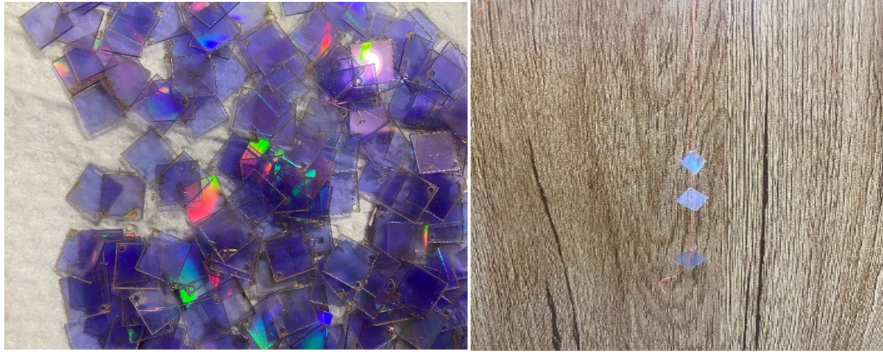
Figure 1: Polycarbonate layer extracted from DVDs.
