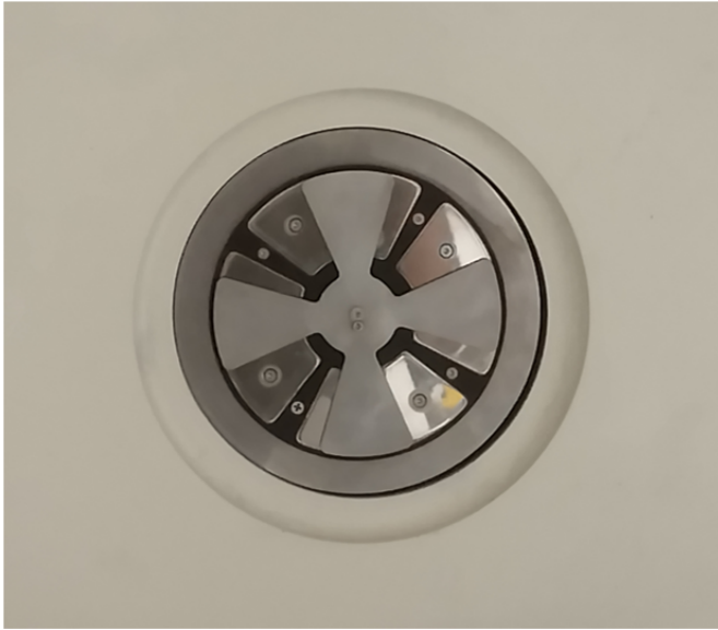
Figure 8: Shutter-Type Generating Voltmeter (GVM).
