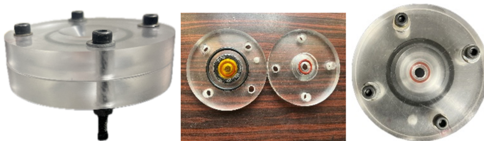
Figure 2: The support is made to place the source inside the water.
