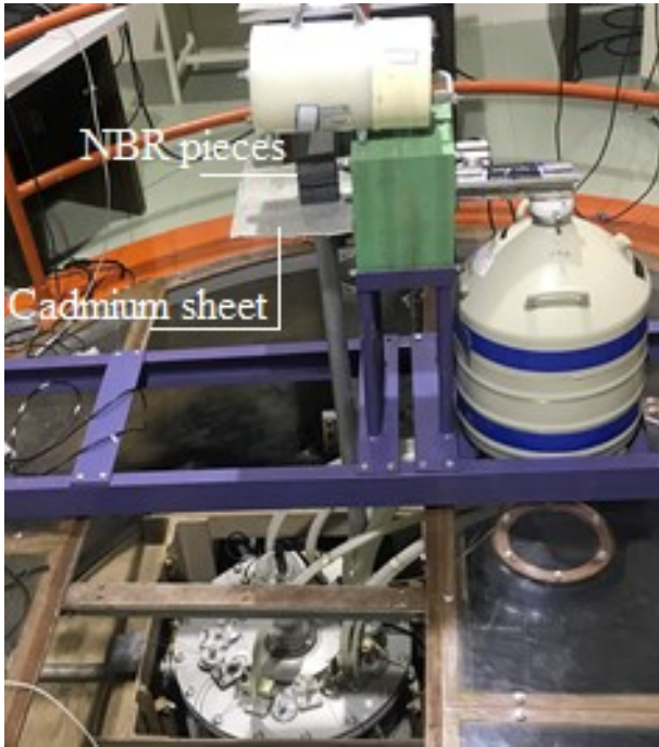
Figure 6: The 6 \times 6 \text{ cm}^2 cutted NBR sheets and cadmium sheet top of MNSR vertical beam line.
