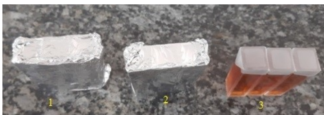
Figure 2: Classification of the cuvettes into three groups (1) stored in the dark and refrigerator (2) stored in the dark and room temperature (3) stored in light and room temperature.
