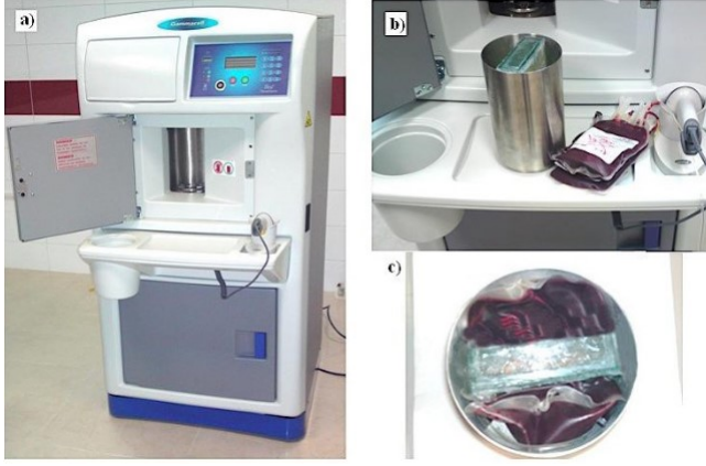
Figure 2: The gamma blood irradiator (a), gel phantom (b), and gel phantom inside the blood container ready to be irradiated (c) (Mohammadyari et al., 2014).
