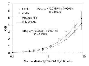
**Figure 4:** Calibration curves of the film badge under Cd-Pb and Sn-Pb filters irradiated by the mixed field in Isfahan MNSR.
