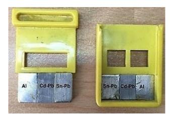
Figure 1: Picture of AERE/RPS badge with Cd-Pb filter embedded in the both sides.
