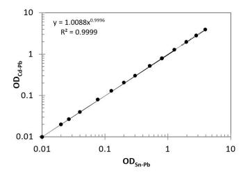
**Figure 3:** Variation of the film optical density under Cd-Pb filter vs. the optical density under Sn-Pb filter. The film has similar sensitivity to gamma rays under these filters.
