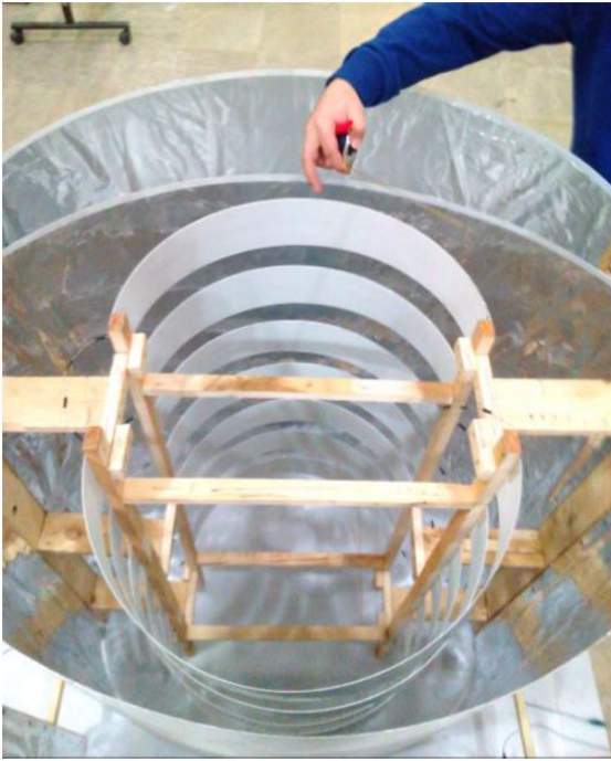
Figure 3: A proof-of-concept model of a parallel-fed capacitive coupled voltage multiplier.
