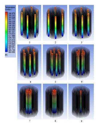
Figure 16: Fluid temperature in core.
