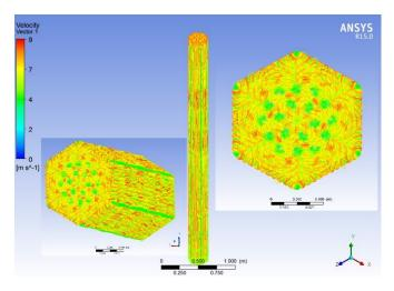
Figure 10: Velocity vectors with crossflows.
