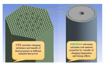
Figure 1: Fuel assembly and Fuel rod in simulation.
