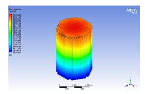
Figure 17: Fluid temperature in full core.
