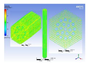
${\bf Figure~11:~ Velocity~ stream~ lines~in~fuel~ assembly.}$
