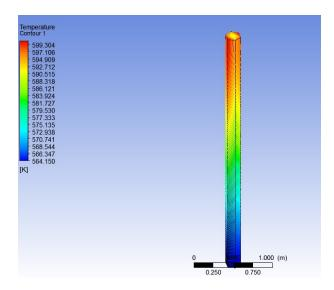
Figure 13: Fluid temperature in fuel assembly.
