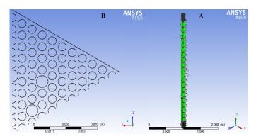
Figure 8: One sixth of fuel assemblies, (A) completely, (B) top view.
