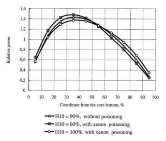
Figure 9: Power axial distribution profile (FSAR, 2005).
