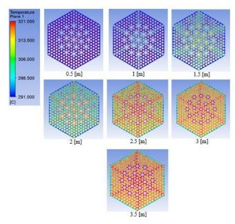
Figure 14: Fluid temperature in different heights of a fuel assembly.
