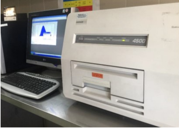
Figure 1: Harsha model 4500 reader used in this project to read dosimeters.
