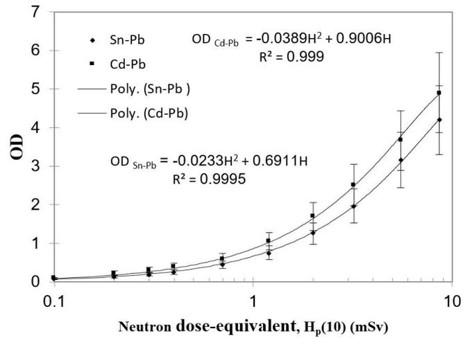
**Figure 4:** Calibration curves of the film badge under Cd-Pb and Sn-Pb filters irradiated by the mixed field in Isfahan MNSR.
