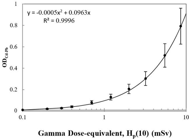
**Figure 2:** Calibration curve of the film badge under Cd-Pb filter irradiated by Co-60 in Karaj SSDL.
